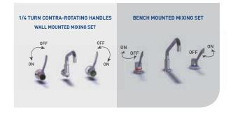
**NOTE:** Diagram for handle rotation reference only - LEVA handles pictured here.
