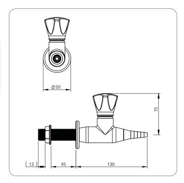
Enware tapware must be installed in accordance with the provisions of, AS/NZS3500 and any relevant local regulations. Installations not complying with AS/NZS3500 may void the product and performance warranty provisions.
