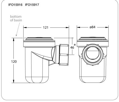
\* Waste outlet height for Micro Trap is 30mm lower than Short P-Trap (IFO14954) that is supplied as standard on all Ifo basins.
