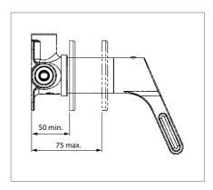
Purge hot and cold water lines, and connect water supply pipework to the hot and cold inlets. Connect the shower outlet to the riser leading to shower rose / outlet.
