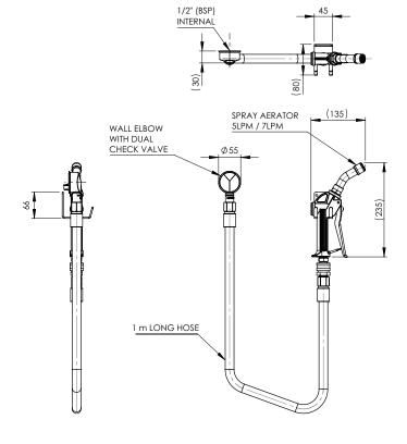
Enware products are to be installed in accordance with the Plumbing Code of Australia and AS/NZS3500. Reference should also be made to the Australasian Health facility Guidelines (AHFG), ABCB and Local Government regulations when considering the choice of, and the installation of these products. Enware Australia advises:
