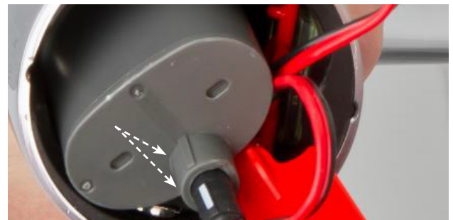
Align white strip with moulded line on battery case
