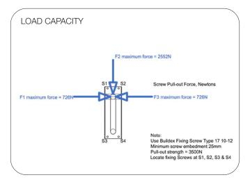
Fixing screws are not supplied with this product. Ensure grab rail is installed on a solid wall surface with firm wall backing using appropriate fixing method. Structural engineers or licensed tradespersons should be consulted for appropriate advice on suitability of the fasteners and wall structure before affixing or installing any Enware products. Enware does not provide any warranty in relation to bolts, screws or other fasteners used with Enware products.
