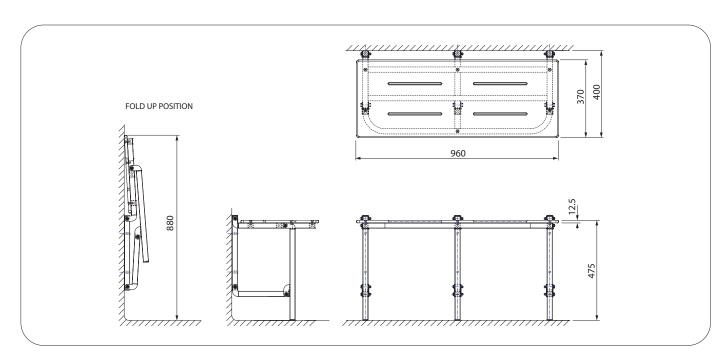
Fixing screws are not supplied with product. Ensure grab rail is installed on a solid wall surface with firm wall backing using appropriate fixing method. Structural engineers or licensed tradespersons should be consulted for appropriate advice on suitability of the fasteners and wall structure before affixing or installing any Enware products. Enware does not provide any warranty in relation to bolts, screws or other fasteners used with Enware products.
