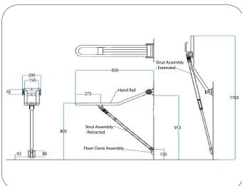
Fixing screws are not supplied with this product. Ensure the product is installed on a solid wall surface with firm wall backing using appropriate fixing method. Structural engineers or licensed tradespersons should be consulted for appropriate advice on suitability of the fasteners and wall structure before affixing or installing any Enware products. Enware does not provide any warranty in relation to bolts, screws or other fasteners used with Enware products.
