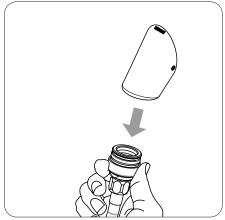
Holding the lock nut, pull the end fitting straight out.
