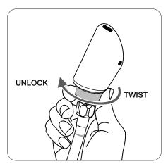
Twist the lock nut anti-clockwise to unlock hand shower fitting.
