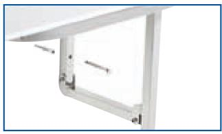
Fixing - Screw wall mount to wall with stainless steel coach screws. Note: On stud wall, make sure wall mount is fixed into studwork and noggins. For masonry walls, use wall plugs supplied.
